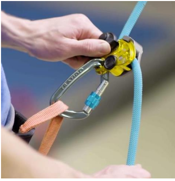
Correct hand position when lowering a climber with a grigri.
