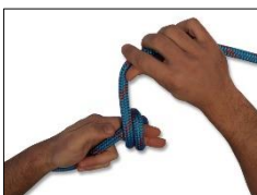
2. Start wrapping the working end around the fingers along and over the standing end.
