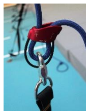
Rope correctly threaded through ATC
