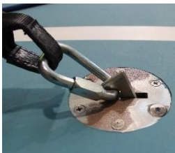
Maillon attaching sling to floor anchor
